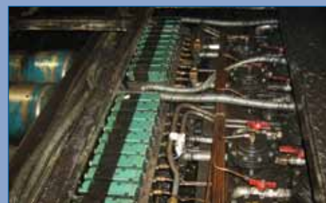
Typical competition solution - Valve with a flow up to 800 NI/min
