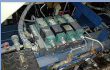
Typical competition solution - Valve with a flow up to 800 NI/min
