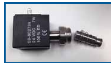
Skinner type pilot disassembled
