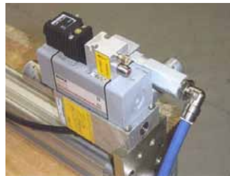
OEM supplied solutions (from left to right): Blow nozzle valve, high pressure pilots, stretch rod cylinder valve
