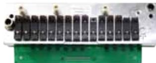
This OEM supplied filling valve control manifold is made of a small solenoid valve driving a spool that is directly built in the manifold. Such a design is prone to leakages, variations in filling levels and the solution has a poor lifetime.
